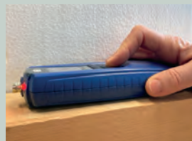
Non-destructive measurement by means of a single-point contact area [LED flashing for limit exceedance]
