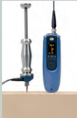
Resistance-based measurement in hardwood using an M 18 ram-in electrode
