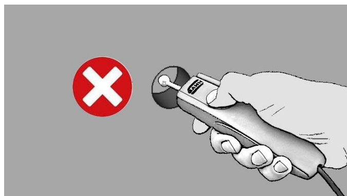
Figure 13-4: Incorrect use – measurement in drill hole
