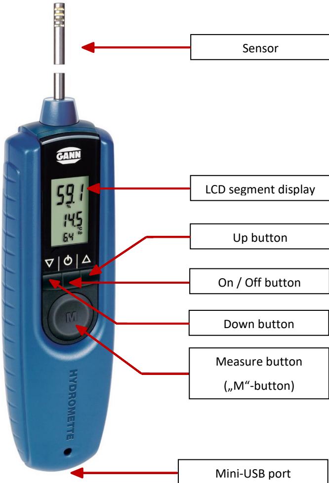
Figure 2-1: View of the Hydromette BL Compact RH-T
