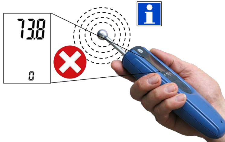
Figure 9-2: Improper device position
