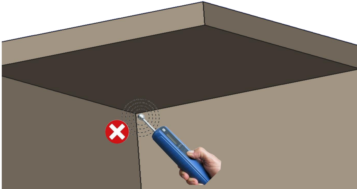
Figure 9-6: Incorrect use in corner/angle area
