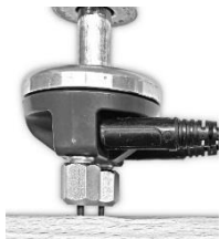
Figure 3-2: Use of Teflon-insulated pins
