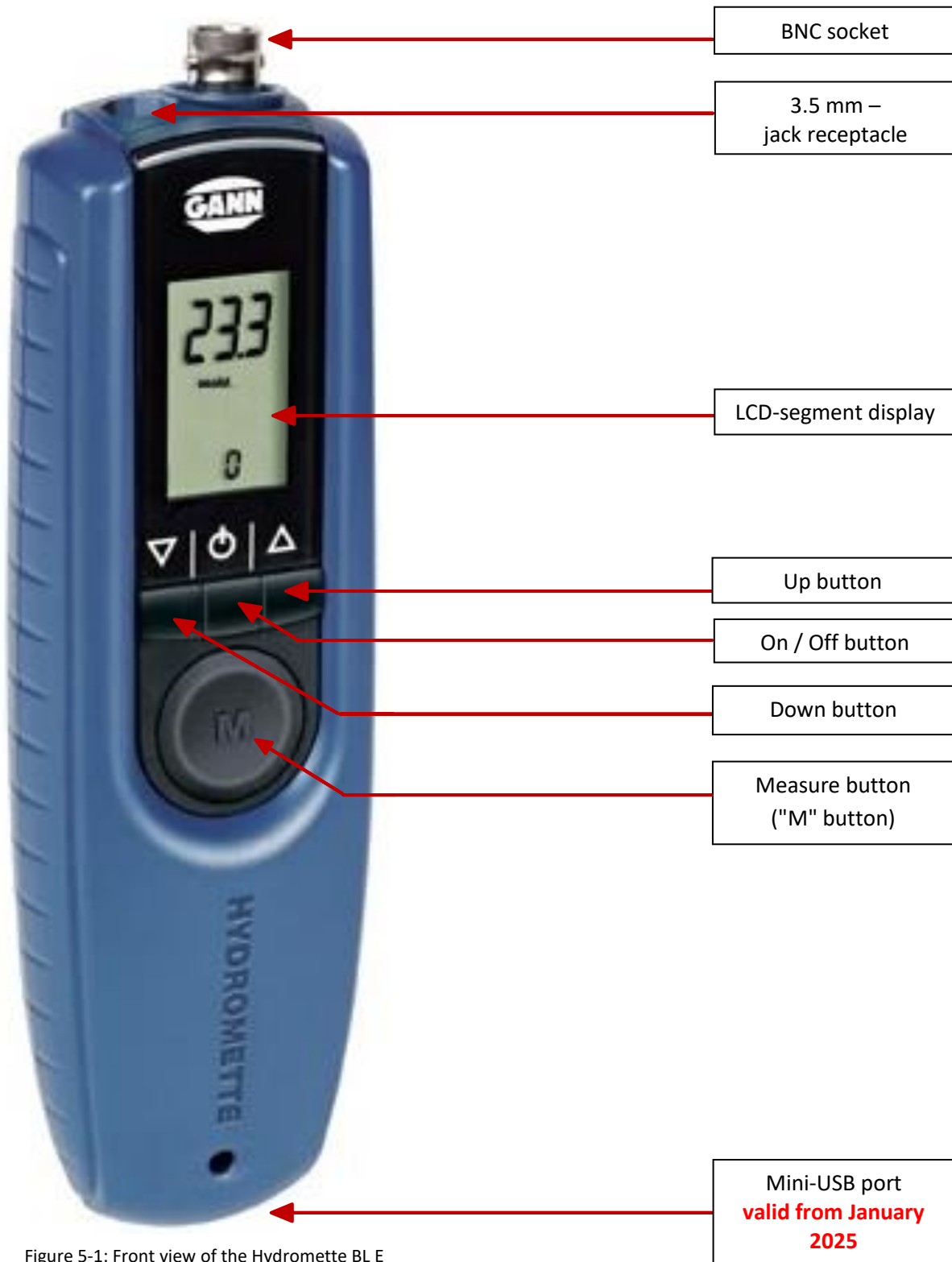
Figure 5-1: Front view of the Hydromette BL E
