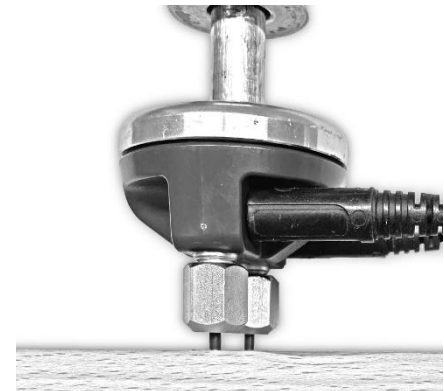
Figure 9-1: Use of Teflon-insulated pins
