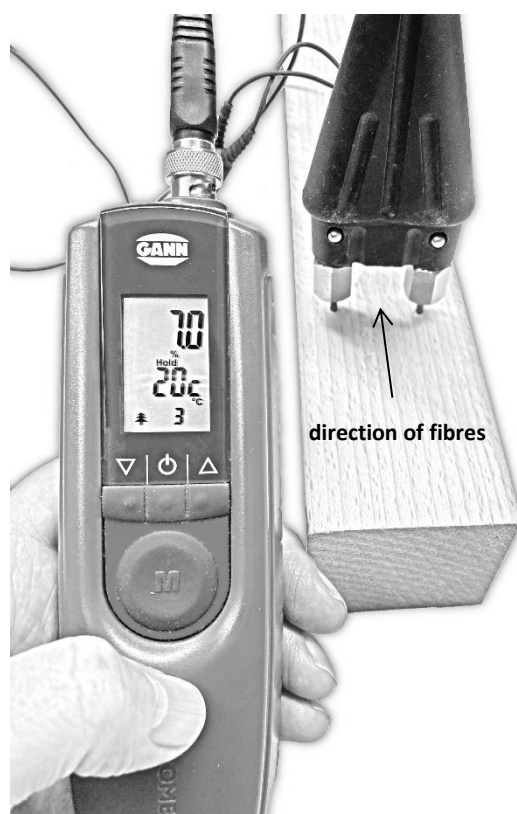
Figure 7-1: Wood moisture measurement – perpendicular to direction of fibres
