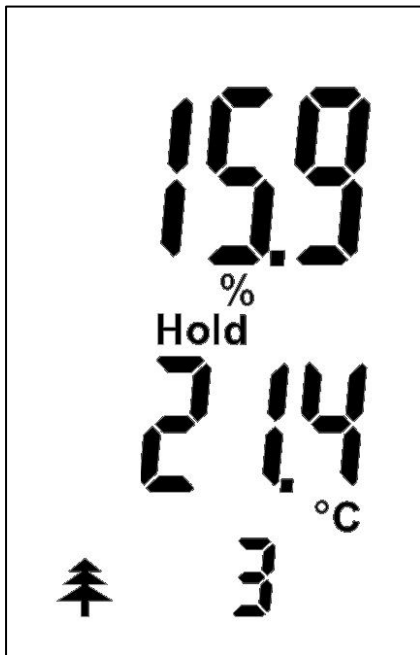
Figure 5-9: Compensation temperature via external temperature sensor
