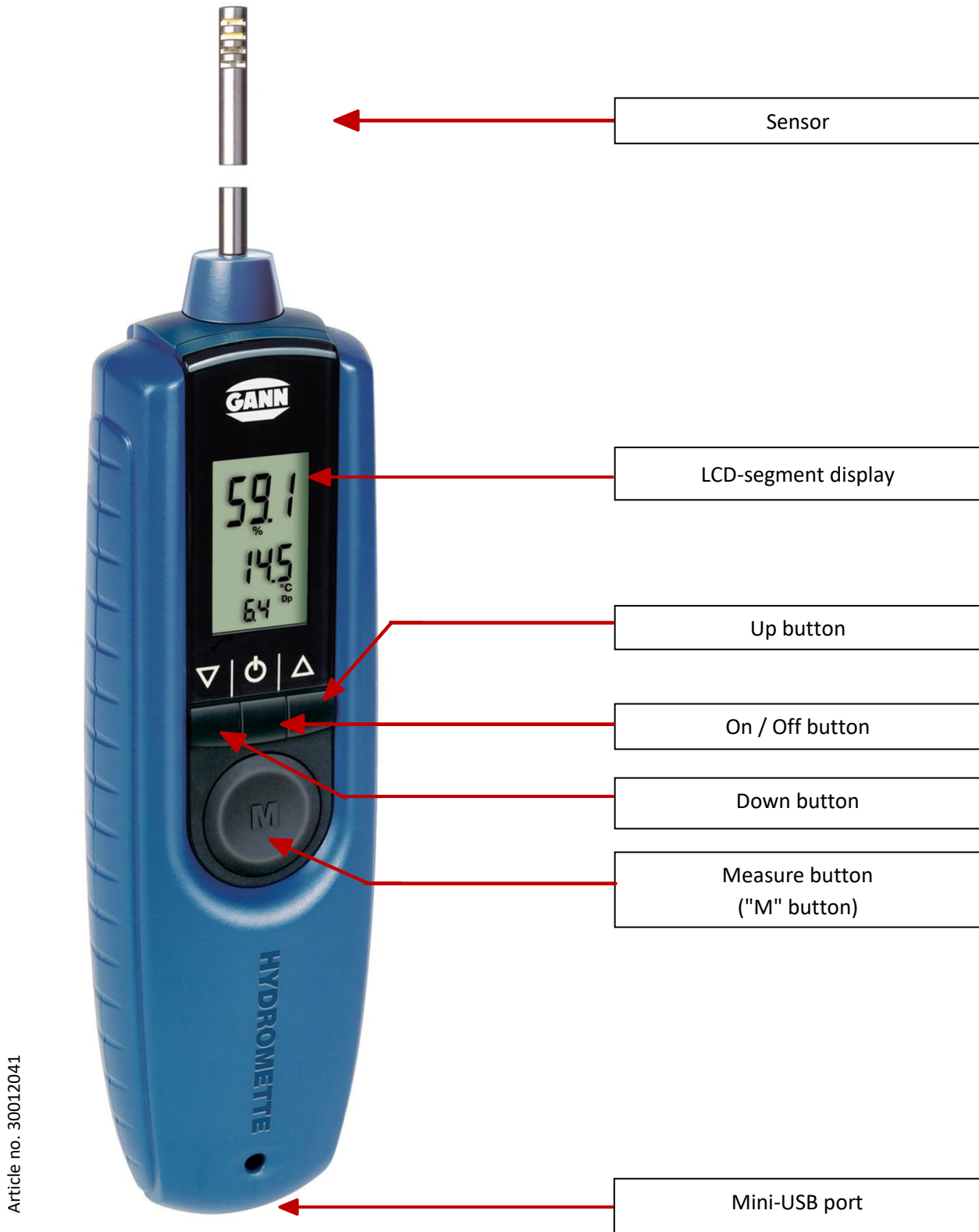
Figure 5-1: View of the Hydromette BL Compact RH-T
