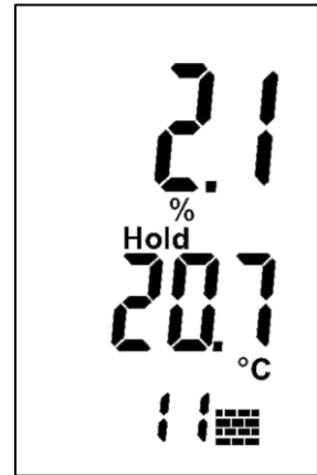
Figure 5-24: Measuring menu "building materials"
