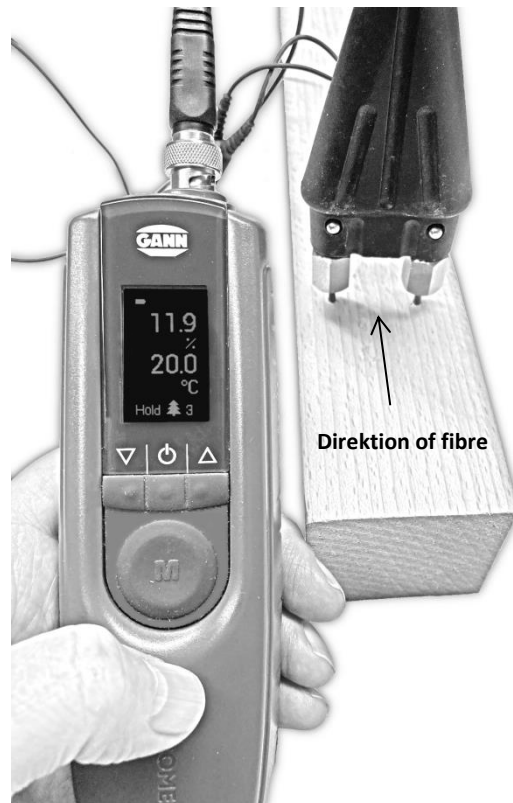
Figure 13-1: Wood moisture measurement – perpendicular to direction of fibres
