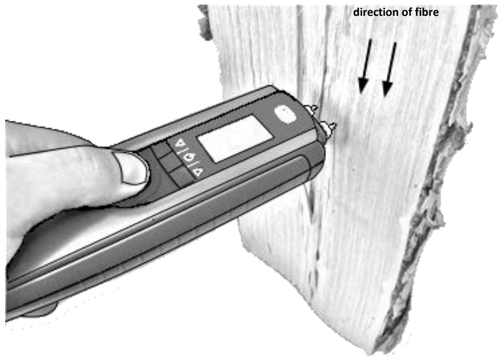
Figure 7-1: Wood moisture measurement – perpendicular to direction of fibres
