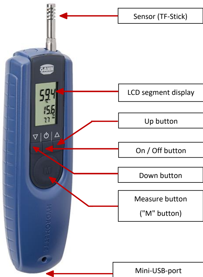
Figure 2-1: View of the Hydromette BL Compact TF 3
