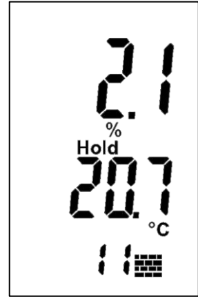
Figure 5-24: Measuring menu "building materials"
