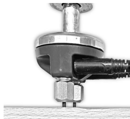
Figure 7-1: Use of Teflon-insulated pins
