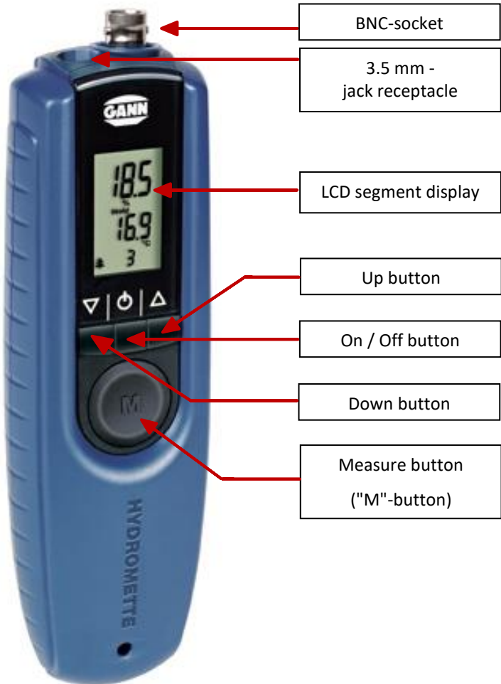
Figure 2-1: Front view of the Hydromette BL HT 70
