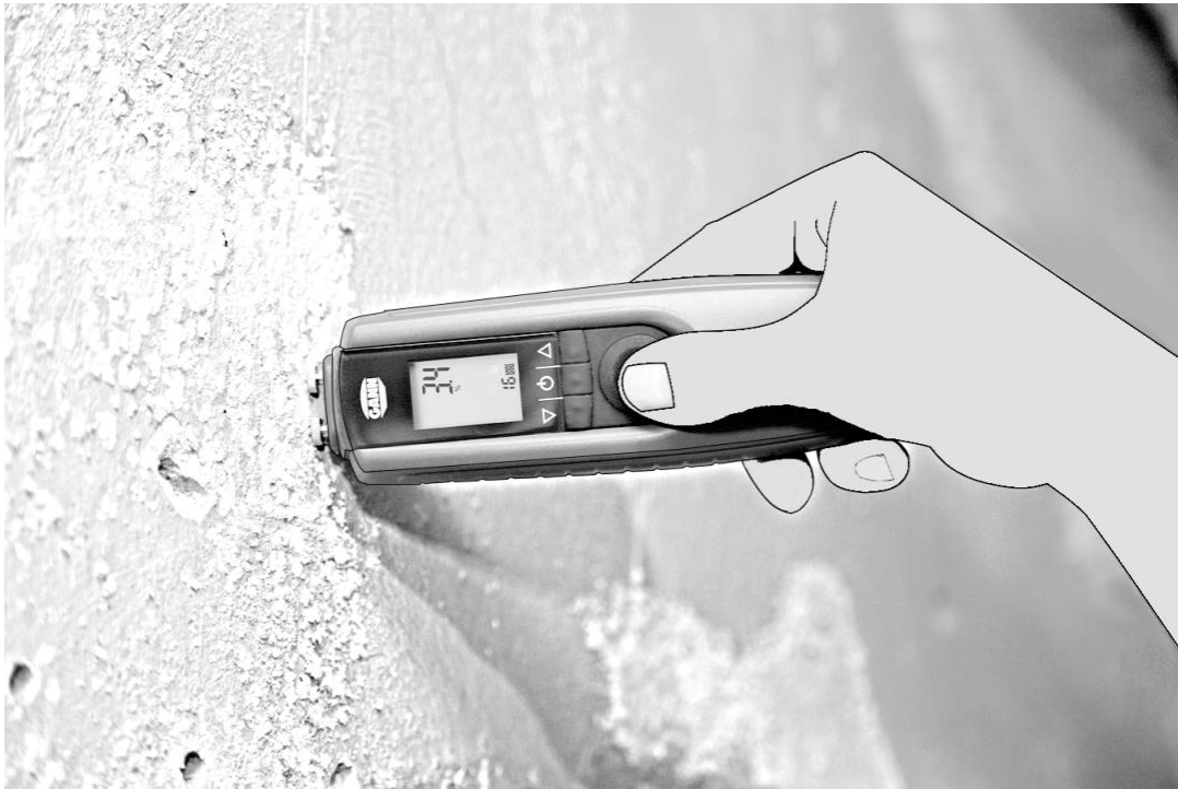
Figure 7-2: Structural moisture measurement – Plaster measurement
