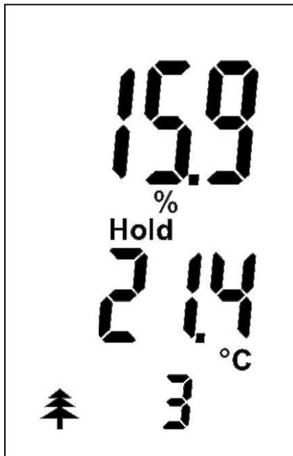
Figure 5-9: Compensation temperature via external temperature sensor
