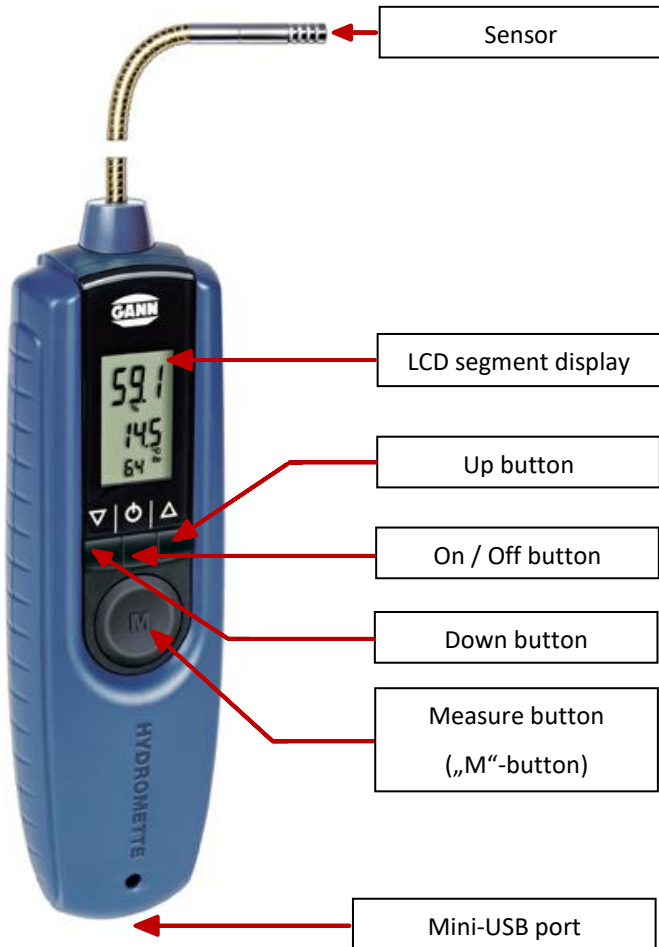
Figure 2-1: View of the Hydromette BL Compact RH-T
